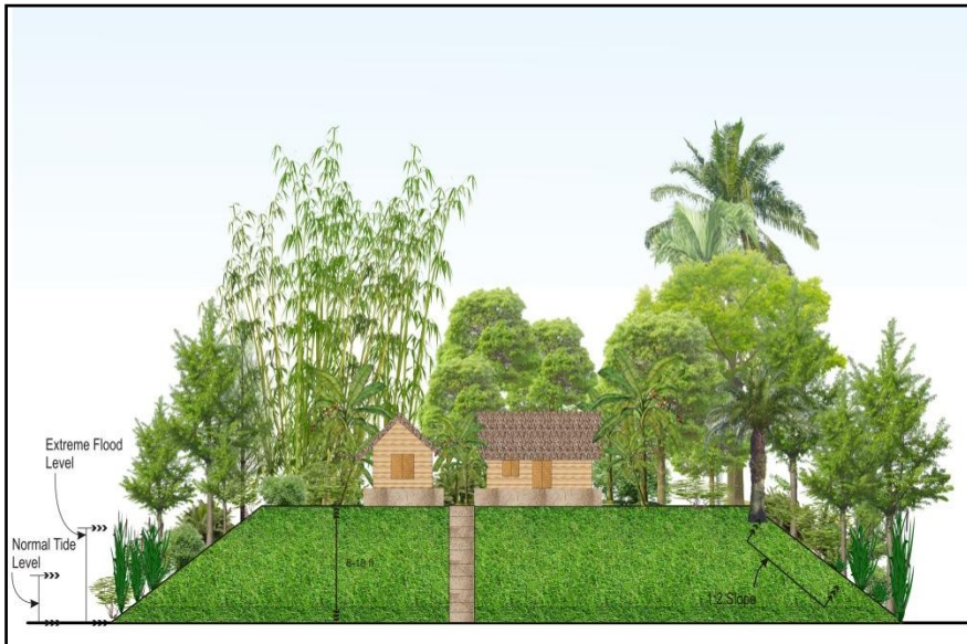
Figure-3: Landscaping of a homestead suited to withstand wind and tide (side view)
