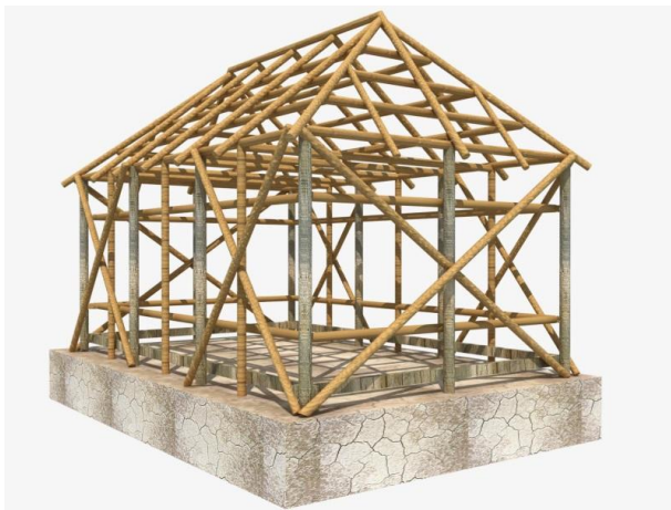
Figure-2: Suggested design of a katcha dwelling house
